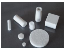
Fig. 1: Flexible geometric shapes of sintered glasses: Tubes, rods, granules and plates were successfully prepared.
