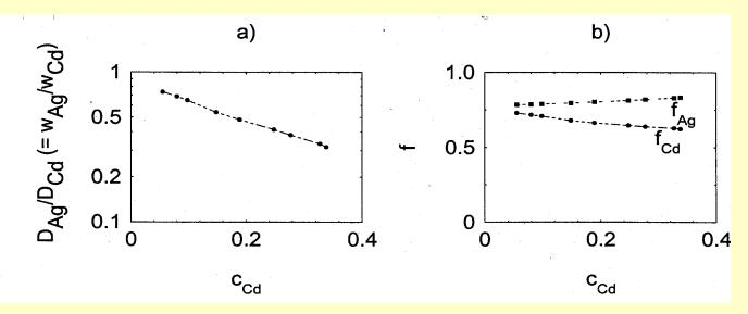
a) The ratio  $D_{Ag}^{I}/D_{Cd}^{I} (= w_{Ag}^{I}/w_{Cd}^{I})$ as a function of  $c_{Cd}$  at 873K. (Iorio *et al.* 1973);
