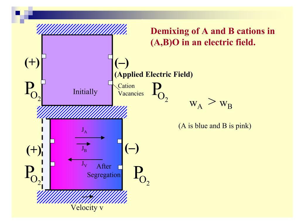
Analysis of demixing of A and B cations in a mixed oxide (A,B)O in an oxygen potential gradient and electric field:
