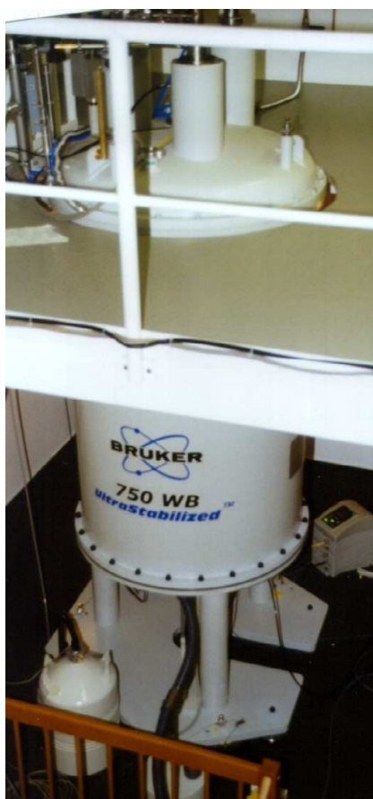
Figure 1: The magnet of the AVANCE 750 with a height of approx. 4 m
