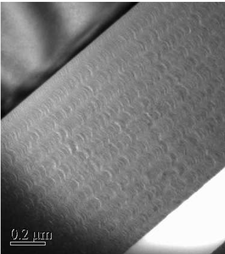
Fig. 1 High-resolution TEM image of a sculptured thin film consisting of \text{TiO}_2 helices, deposited on silicon. (Cross-section and samples are provided with kind support from Prof. Dr. Ian Hodgkinson and Matthew Arnold, Otago University, New Zealand).
