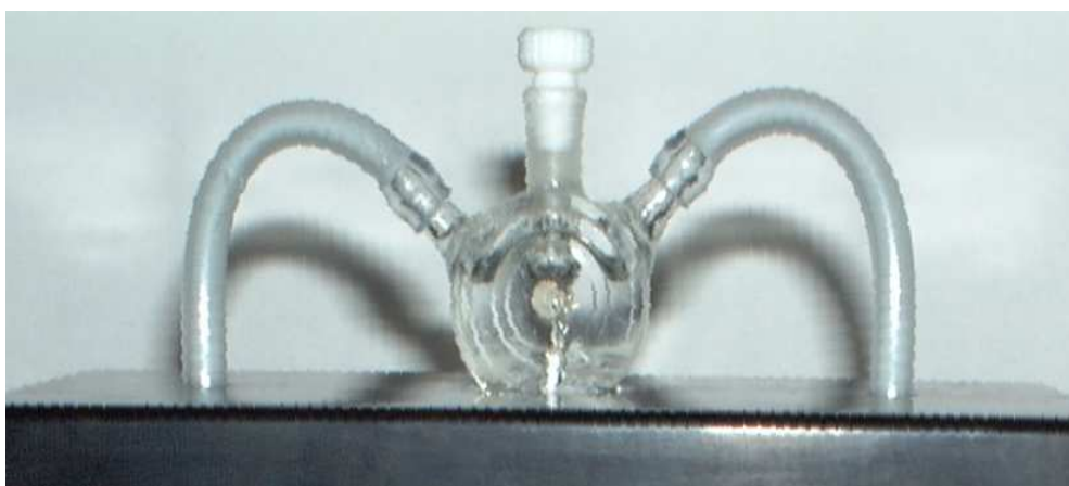
Fig. 3 Miniaturized vessel for 1 ml reaction fluid with ultrasonic transducers at the center of the glass container
