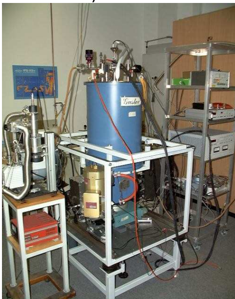
Figure 1: Far infrared ellipsometer at our laboratory with magnetocryostat (Oxford) attached.
