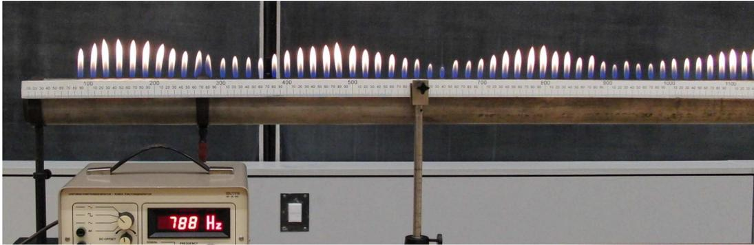
Figure 8.35: Rubens flame tube with fixed end on the left.
