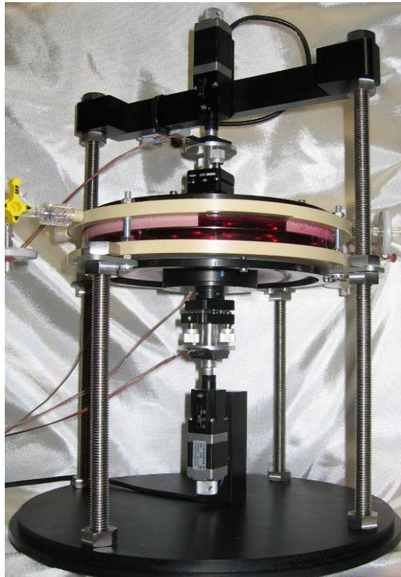
**Figure 9.1:** Bioreactor with integrated non-invasive monitoring for the in situ measurement of ultrasonic and rheological parameters
