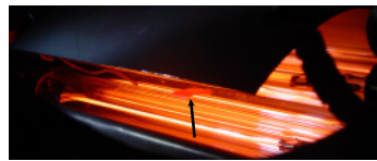
Annealing 2 of ZnO substrate at 1200°C in O 2
