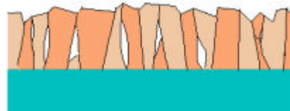
coarse-grain columnar, porous
