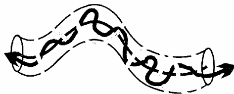
Fig. 7: Modelling the lateral constraints on the chain motion imposed by the entanglements by a "tube". The average over the rapid wriggling motion within the tube defines the "primitive path" ( continuous dark line )
