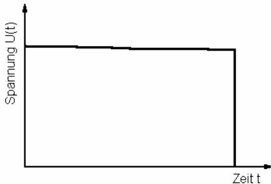
Figure 7: Typical shape of a rectangular pulse (voltage U over time t)
