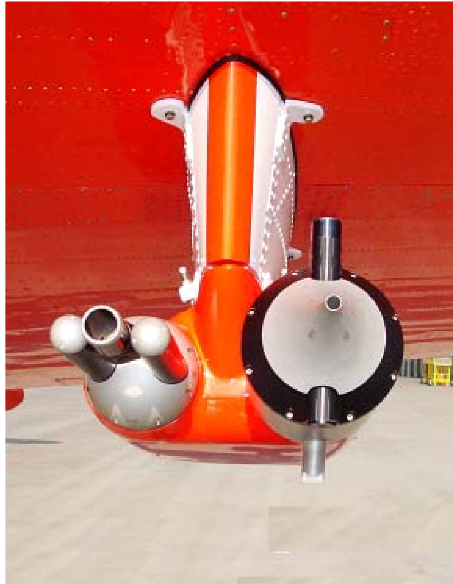
FSSP and Polar Nephelometer installation
