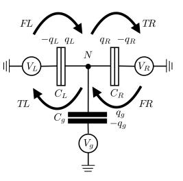
Fig. 1: Capacitance circuit for the single electron transistor with a total of N charges at the central island. The arrows correspond to the four different transfer processes of a single electron with respect to the central island: FL from left, TR to right, TL to left, FR from right.
