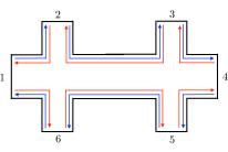
Figure 1: In the quantum spin Hall effect, charge transport is due to onedimensional channels propagating along the sample edges. The spin of the electrons is tied to their motion: left moving (red) and right moving (blue) electrons have opposite spin polarization. The edge channels connect neighboring terminals.
