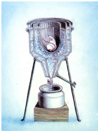
first calorimeter by Lavoisier
